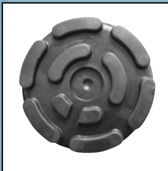
Rubber pad Ø145 mm for lift stabilizers SBR, black, SH 75 A Internal Ø120 mm Height 24 mm
