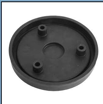
Rubber pad Ø120 mm for lift stabilizers SBR, black, SH 75 A Internal Ø108 mm Height 26 mm
