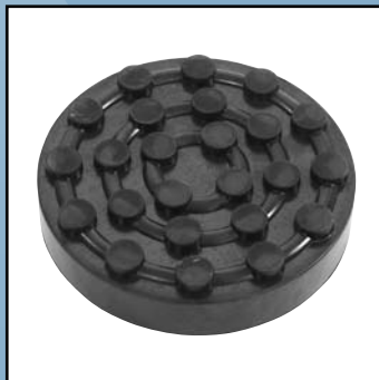
Rubber pad Ø120 mm for lift stabilizers SBR, black, SH 80 A Internal Ø108 mm Height 26 mm
